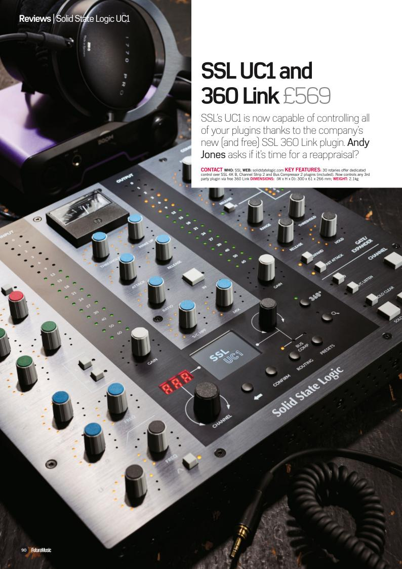
SL's UC1 controller was released around three years ago, and is a direct knob-per-function interface for controlling the SSL Channel Strip 2, 4K B and Bus Compressor 2 plugins.
