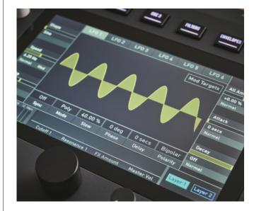
selected on either side, while the applied modulation amount can be dialled in as either a positive or negative value. However, one of the crowning glories in the modulation stakes is the Komplex Modulator, which allows the user to create very complex modulation shapes, right on the touchscreen. Armed with a full 40 modulation slots, you're therefore unlikely to run out of modulation options very quickly.
