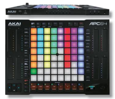
PADS: 64 RGB backlit pads with velocity and pressure sensitivity. Expanding the grid from 5x8 is good news for melodic players
