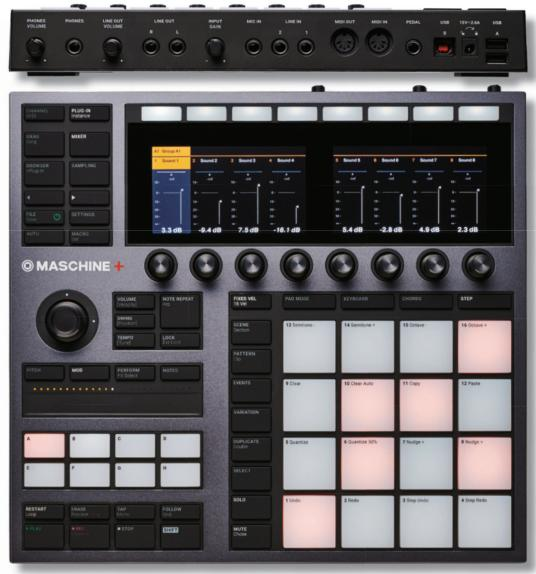
LAYOUT: Slight changes to button labels aside, the top panel controls are identical to the Maschine Mk3's
