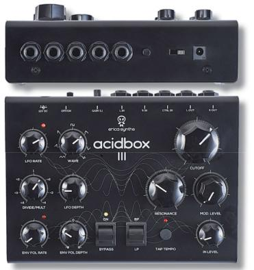
**CONTROL IN** The rear panel control jack can accept foot switches, expression pedals, trigger inputs or CV modulation. MOD LEVEL The global modulation depth rotary is handy for punching or fading in modulated effects. **INPUT LEVEL** The front panel level control is actually more of an overdrive, imparting a lovely, gritty distortion.
